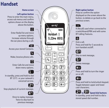
The answer machine handset controls on buttons 2\* 4° 5 and 6 will only work when a message is being played on the handset.
