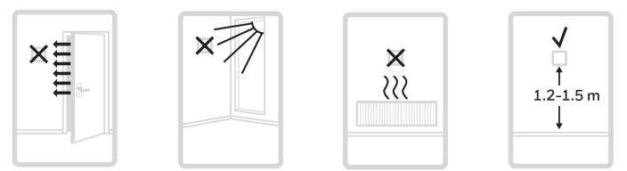
The T6R thermostat should not be placed near draughts, in direct sunlight or near heat sources. It should be at least 1.2 - 1.5 meters from the floor.
